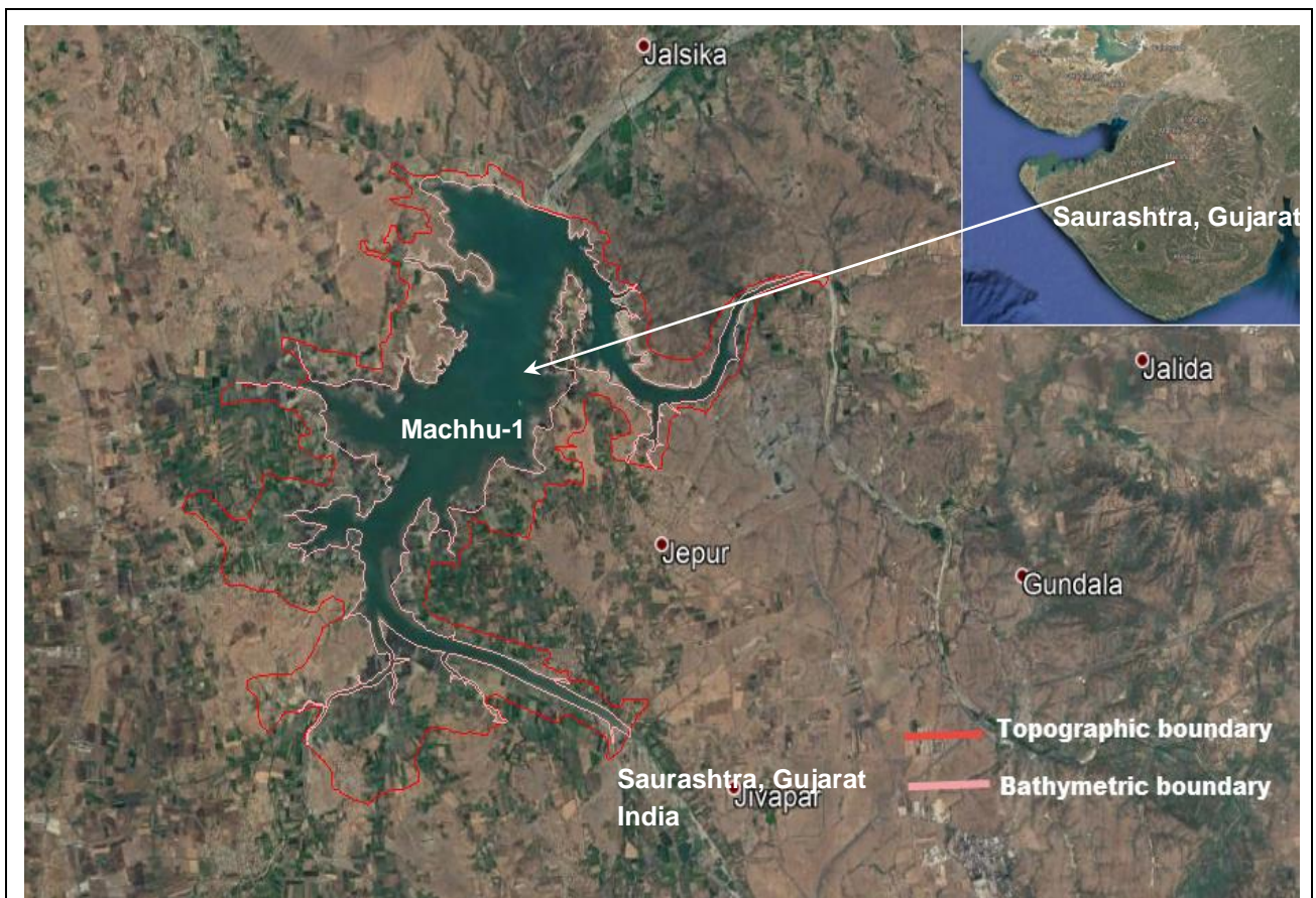
Figure 2: Surveyed areas (Topographic and Bathymetric) – Machhu-1 Reservoir
